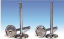
We also stock the range of Paul Ivey developed Rimflo valves for the A-Series. They are made of EN214N steel with chrome plated stems which enable them to be used with standard iron guides.
