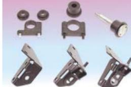
For alteration of the rear camber there are three types of radius arm bracket. First is a fixed set that adds 1 1/2° of negative camber to whatever the car has with standard ones. The second is adjustable to allow preferential settings to be reached. The third is adjustable for both camber and toe.
