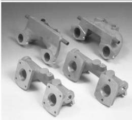
The twin SU manifolds have been carefully produced to minimize cross-port-flow interference caused by the balance tube, and have good radiuses in all the right places. Further blending can be carried out if required, but leave a ground finish to promote, fuel atomization. DO NOT POLISH!
