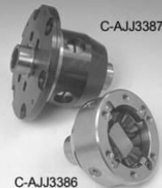
The ultimate in reliability for street and race use. Twice the strength of a stock differential. Contains four spider gears and two cross pins. The greater number of gears means greater reliability since each gear only takes on 1/4 of the load instead of 1/2. The outer cage is also made from billet steel instead of cast. The cross-pin differentials also use stock crown wheels and outputs shafts (not included).
