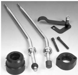
A recent development is the quick shift gear lever kit. It has been designed to reduce the overall gear lever ratio from 8 to 1 to 4 to 1, thereby reducing the distance the lever has to be moved for gear selection.
