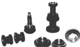
Six variations of all synchro gear sets are available, 3 helical and 3 straight cut. The early standard helical ratio set was fitted to all small bore Mini's, recognizable by their square top teeth. The first motion shaft uses 17 teeth, and the laygear is usually numbered 22G927.
